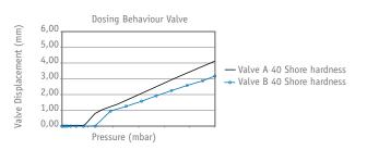
WP developed a proprietary silicone valve solution with a patented technique. The silicone material has a memory for long term seal quality and the opening/closing mechanism. Good temperature resistance is another advantage to give excellent dispensing opportunities for a wide range of viscosities and product applications.
