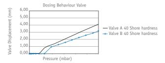
WP developed a proprietary silicone valve solution with a patented technique. The silicone material has a memory for long term seal quality and the opening/closing mechanism. Good temperature resistance is another advantage to give excellent dispensing opportunities for a wide range of viscosities and product applications.
